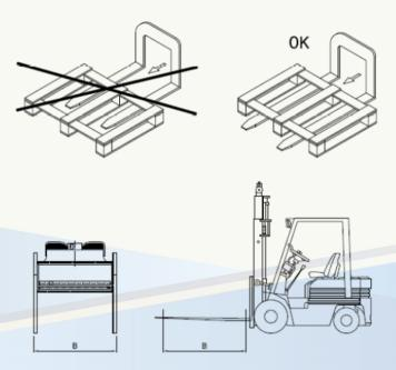
All handling equipment must be chosen according to the weight and the packaging shape of what is going to be handled, the product must be hooked up with appropriate hooks and, if provided in specific documents, only by the points indicated by WingFan S.r.l.
