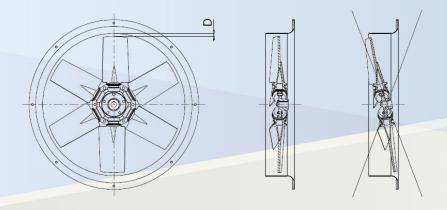
Check that the tip clearance (D) in operation between the impeller and the frame is uniform along the circumference to avoid contacts and rubbings between the impeller and the frame and is at least 0.5% of the frame diameter.
